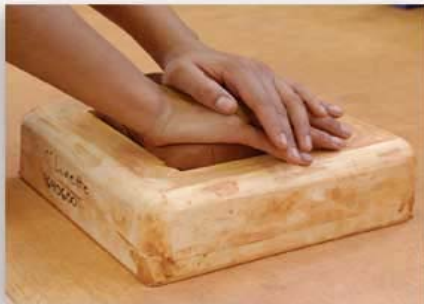
Clay is pressed into a plaster mold
