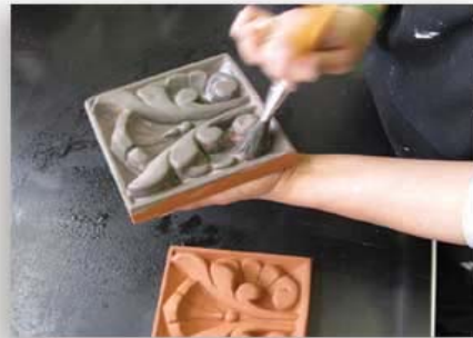
Tile is glazed with a brush after drying and bisque firing
