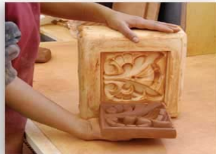
Clay shrinks slightly and is removed from mold
