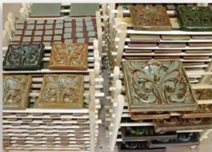
Tiles on special racks after glaze-firing
