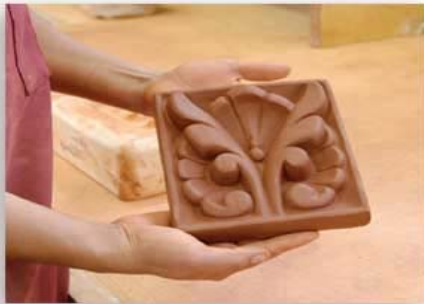
Completed greenware tile ready for drying
